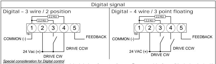
In this mode, the actuator is sensitive to induced electrical voltages **from external sources**. To prevent such interference, if the signal on pins 4 and 3 on TB1 are from an **external 24 Vac source**, install a resistor 2.2kohm, 0.5W between pins 4 and 1 and another of 2.2kohms, 0.5W between pins 3 and 1 of TB1. These resistors are included.
