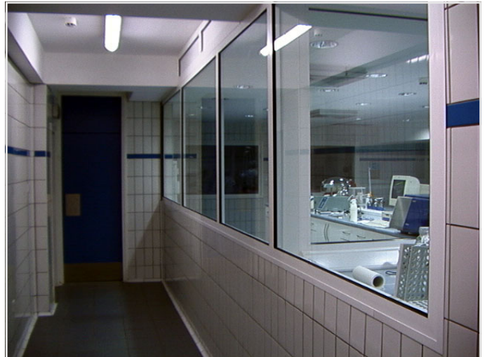
Outside microbiology Laboratory under-pressurized compared with the Lab.
