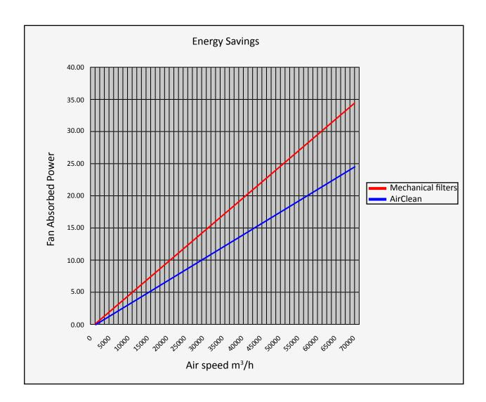
The reason why there is such a difference in pressure loss between the systems depends on the space between collection plates in the electrostatic filters that are not generating significant pressure losses.
