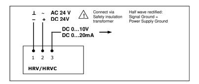
Measuring Signal Humidity. Select Signal type with JP1 The signal range is adjustable with OP THP.
