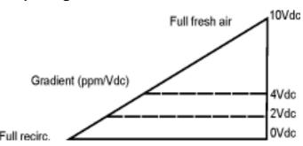
Normal operation is to set dampers to minimum fresh air at below 2Vdc.
