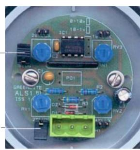
Light level selection jumper (shown in 0-2000 lux mode)
