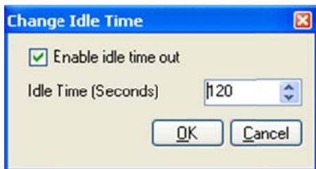
Removing the tick the Enable Idle Time Out box disables admin timeout feature. The timeout value can also be changed.
