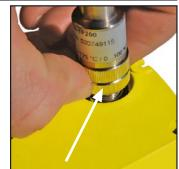
For mounting the probe plug the socket and screw on the sensor by turning the lower knurled thumb clock wise. Just screw hand tight. A small clearance between ExCos-D (transducer) and ExPro-C... (probe) has to be accepted due to production conditions.
