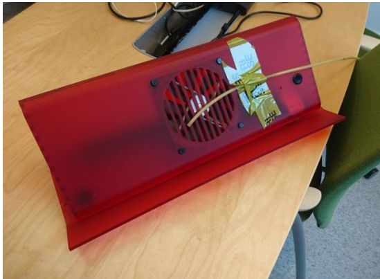
Fig. 1 Exterior of ionization unit, with tubing for measurements of ozone positioned at fan outlet
