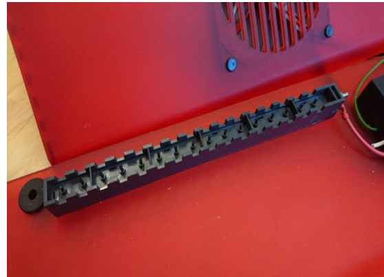
Fig 2. Vital part inside the unit, the 16 carbon brushes air ion generator rod; "SPG"
