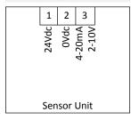
The detector is supplied with a 2-10Vdc control signal.
