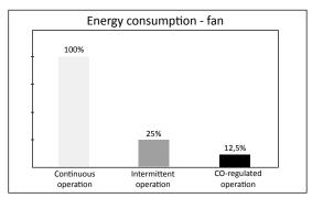
By monotoring CO levels and only running the fans when necessary the CO detector becomes a significant energy saver.
