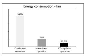
By monotoring CO levels and only running the fans when necessary the CO detector becomes a significant energy saver.
