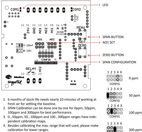
5. Before any calibration, check CONFIG Jumpers and set to calibration level.
